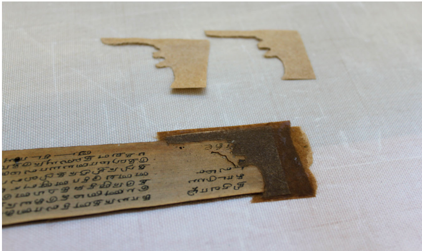
Fig. 11 Infills being applied to a palm leaf manuscript with wheat starch paste by building up layers of Japanese paper to reach the desired thickness.
